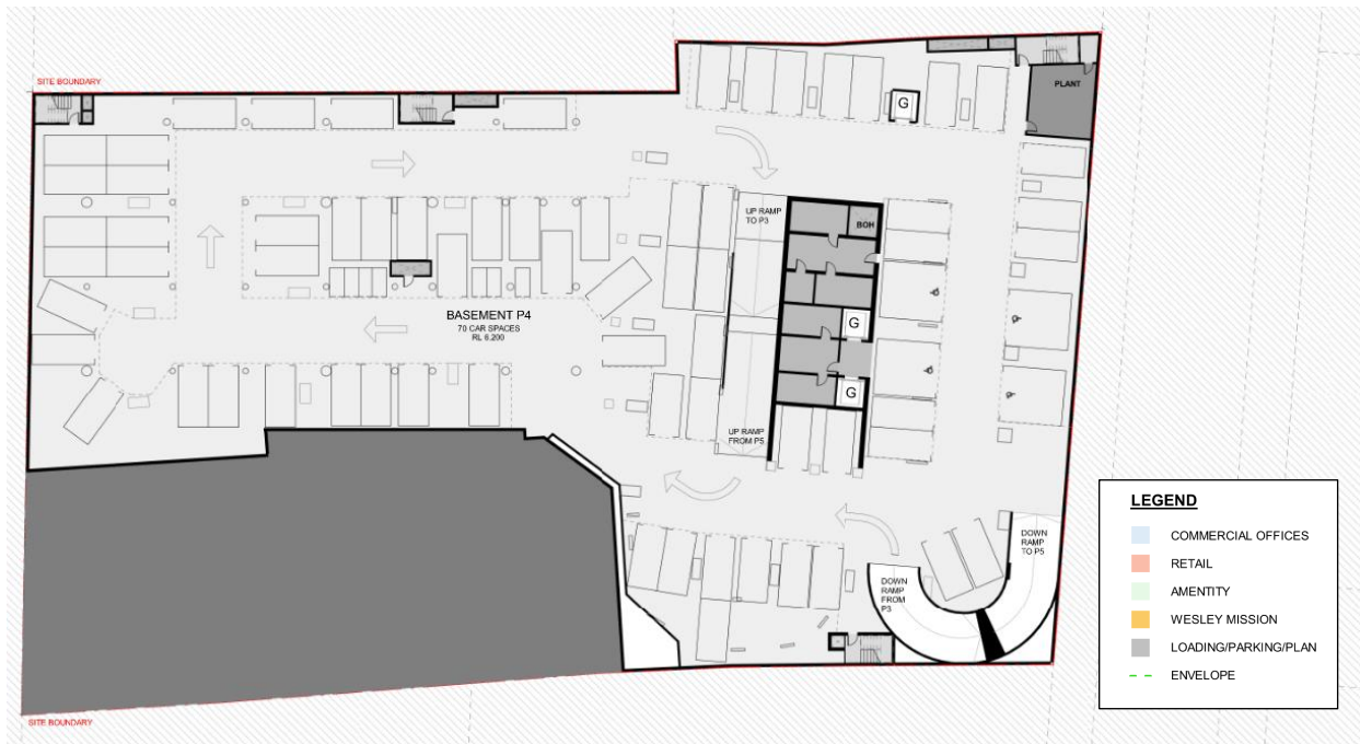
Figure 15: Parking layout - Level P4.
